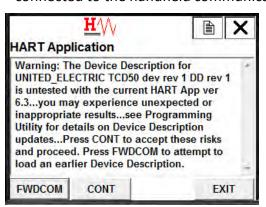
This is a standard warning for any unregistered DD and should not effect Vanguard operation or data reporting.
