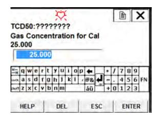
Desired gas concentration value is saved into the Vanguard device.
