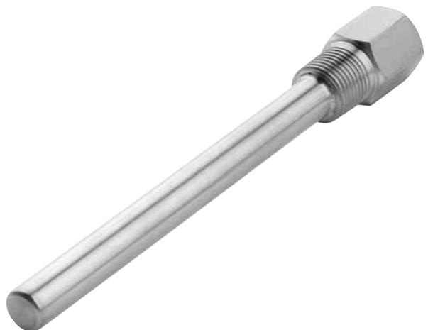
Thermowells are used to protect the measuring instrument from corrosion, high pressure or high fluid velocity and to allow the measuring instrument removal for recalibration or replacement without affecting the process system. The W10-W20 serie includes thermowells with threaded process connection. These thermowells are suitable for low/medium work intensity.
