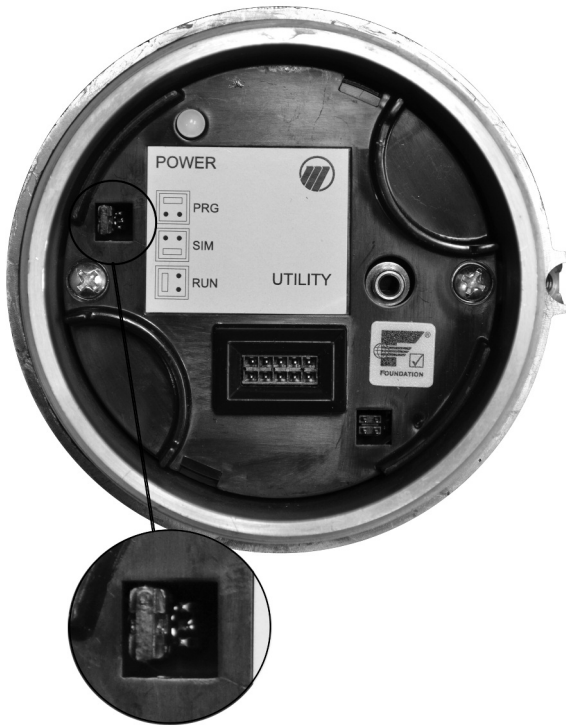
Remove jumper to disable simulation
