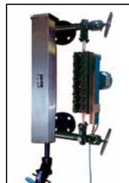
LevelMax unit with Flat Glass gage lit by DuraStar Illuminator. Optional low to medium pressure models are rated up to 1500 PSI (100 Bar) with lever actuated water gage isolation valves and an end stem connected water gage for easy maintenance.
